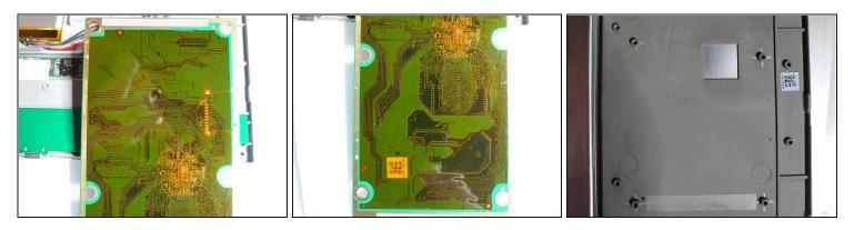
• Interestingly, even the other side of the mainboard contains some elements near the CPU which require a semicircle hole cut into the frame... interesting design decision.
