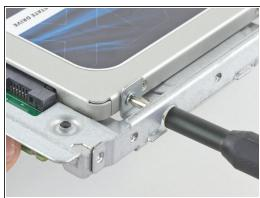
Use a Phillips screwdriver to install the four silver screws (two on each side) along the edges of the SSD to secure it to the enclosure.
