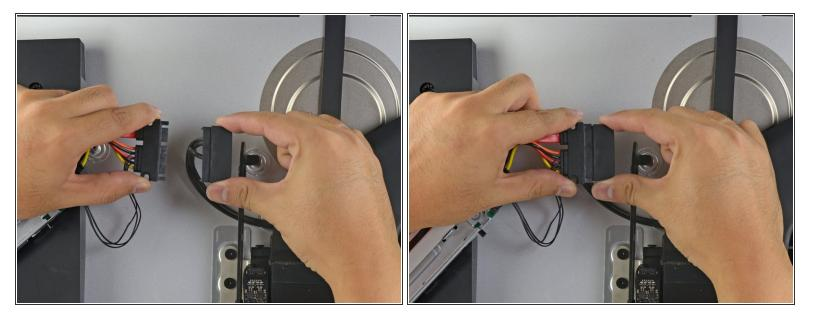
• Connect the iMac's combo cable to the new temperature-enabled combo cable.
