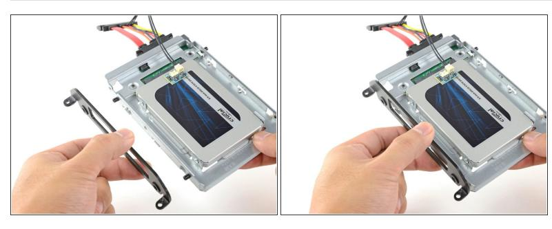
Attach any mounting brackets removed from the old hard drive onto the enclosure.
