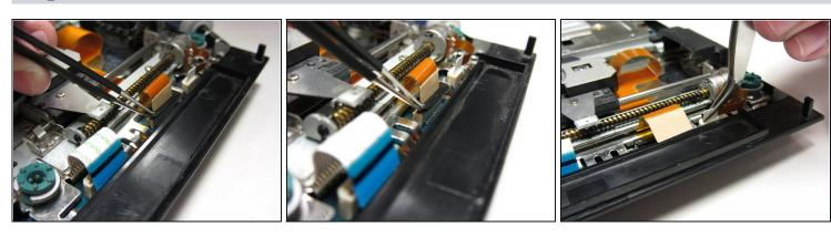
• Using <u>tweezers</u>, gently detach all three ribbons from the motherboard terminal. Unlock the middle orange ribbon to lift the black tab up on either side.
