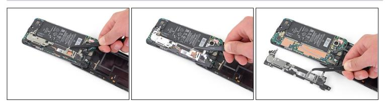
• Use a pair of tweezers to remove the motherboard bracket.
