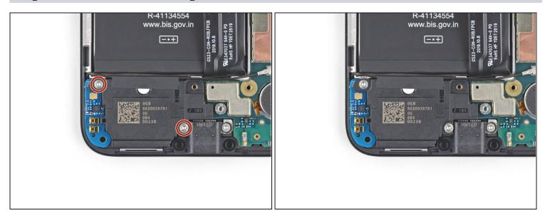
Use a T3 Torx driver to remove the two 4.1 mm screws securing the loudspeaker assembly.
