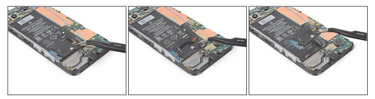
Carefully peel the loudspeaker assembly up off of the tape underneath it.
