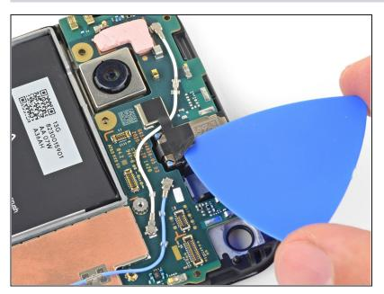
Use the corner of an opening pick to peel up the tape covering the earpiece speaker.
