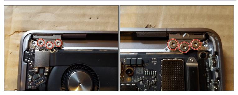
• Use a T9 Torx driver to remove the six 4.7 mm screws securing the display hinges to the upper case.
