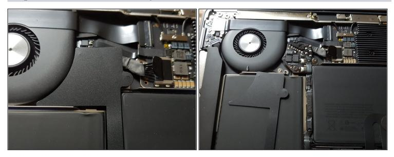
• Remove the plastic shield covering the battery PCB.
