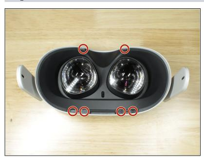
Start by removing the six T2 screws that hold the inner lining of the headset to the front.
