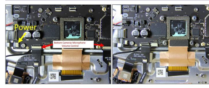
Open the flaps on the 3 ZIF connectors and detach the ribbon cables.
