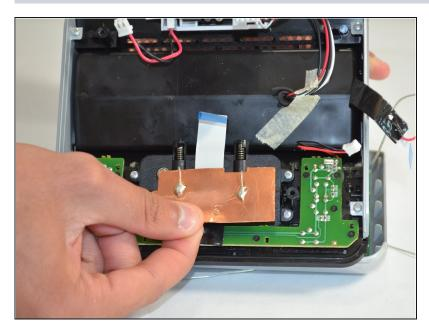
Pull the copper plate out of the way of the two Phillips #00 screws in the middle of the connector.
