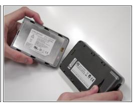
Push the black button and slide the battery casing to the left simultaneously, until the battery is completely separated from the device.
