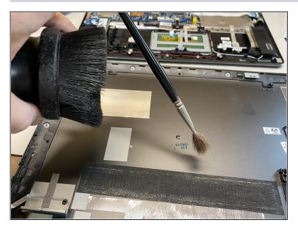
• It's amazing how much dust and debris can find its way into a computer over time, drawn in by the cooling fan. The more that builds up the more likely it is to overheat. Thus it's a good idea to use either a small soft brush and vacuum or compressed air to gently remove as much dust as you can before reassembly.
