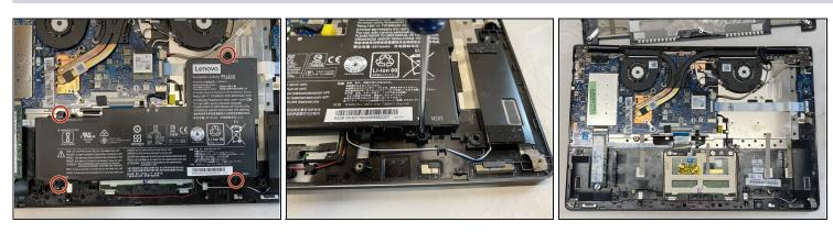
• The battery is held in place by **four identical #1 Phillips head screws**. Remove each of these and then carefully lift the old battery out. Recycle appropriately.
