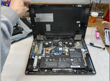
• In addition to the ten screws, the back is held in place with a number of **small plastic tabs**. Starting at one corner, carefully pry the back of the case off. I found using a small flat screwdriver (or spudger) and a guitar pick makes this easier as you work around the four sides.
