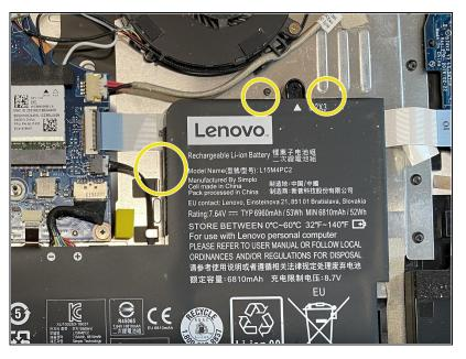
When installing the new battery, I found it easier to plug in the connector prior to screwing the battery in place. Also, ensure the battery clears the small aluminum locator tabs around the sides.
