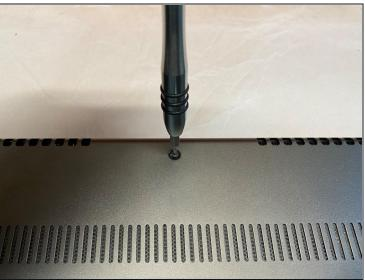
• Using a Torx T5 driver, remove all ten screws securing the back of the case. **Note that the three screws closest to the hinge side are longer than the others.** Putting these in the wrong location when reassembling could damage the laptop.
