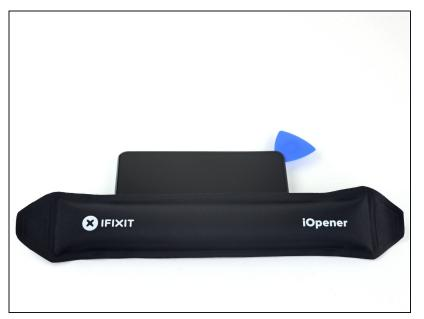
Apply a heated iOpener to the left edge of the screen for one minute.
