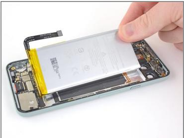
⚠ Do not reuse the battery if it has been deformed or damaged, as doing so is a potential safety hazard. Replace it with a new battery.
