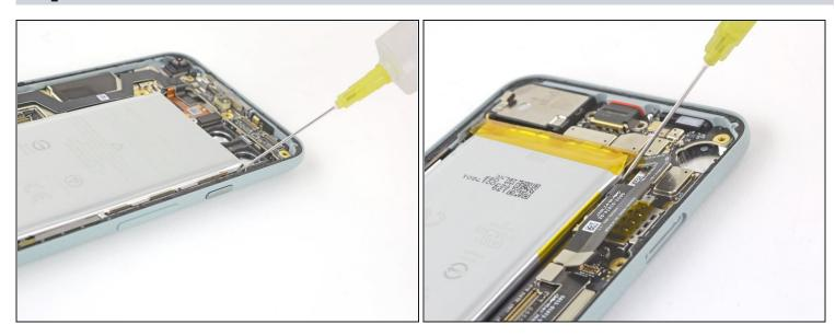
• If any of the adhesive strips broke off underneath the battery and could not be retrieved, apply a few drops of high concentration (over 90%) isopropyl alcohol into the opening of the affected tab.
