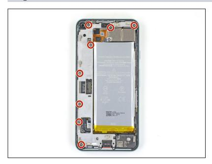
Use a T3 Torx driver to remove the eight 4.6 mm-long screws securing the midframe.
