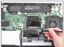
• Use the spudger to slide the battery socket connector parallel to the motherboard and out of its socket on the motherboard.
