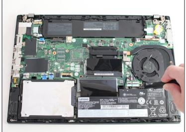
Using the Phillips #1 screwdriver, remove the two 4.6 mm screws securing the internal battery to the frame.
