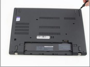
Using the Phillips #1 screwdriver, loosen the six captive screws.
