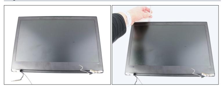
Use the metal spudger to create a space between the bezel and lid and carefully undo the clips around the perimeter of the bezel.
