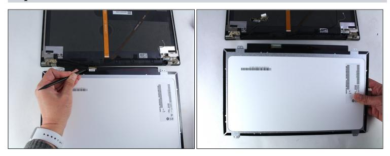
• Using the black nylon spudger, disconnect the display connector cable and remove the LCD screen.
