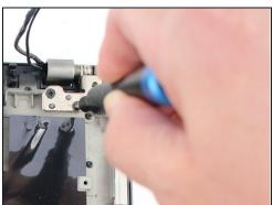
• Using the Phillips #1 screwdriver, remove two 4.3 mm screws from each hinge (four total).
