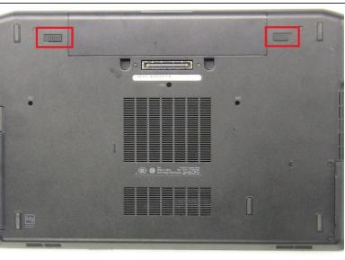
Make sure your computer is unplugged and off before removing the battery
