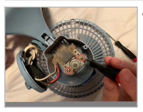
Remove two 38.1 mm Phillips #2 screws from the motor.
