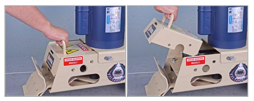
• Pull the hood away from the device to remove it.
