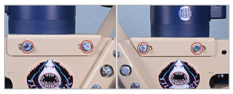
Use a 9/16 inch socket to loosen, but not remove, the four bolts securing the motor mount to the frame, two on each side.
