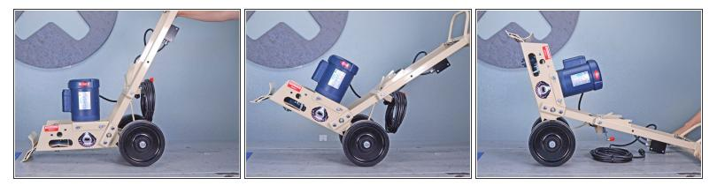
• Tilt the device back to rest on its handle.
