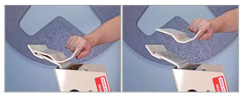
• Remove the blade retainer.
