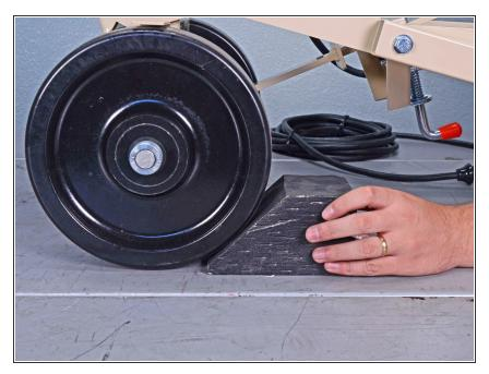
Insert wheel chocks behind the wheels to ensure the device does not move or fall during the repair."
