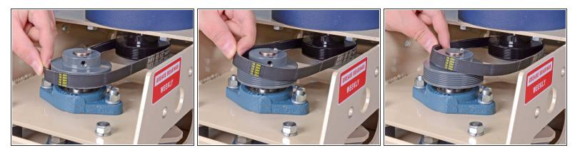
• Remove the belt from the cam shaft pulley.
