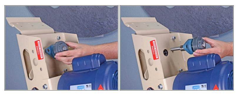
• Remove the cam shaft assembly
