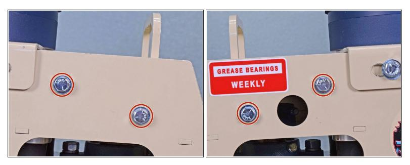
Use a 1/2 inch socket to remove the four bolts securing the hood to the frame, two on each side.
