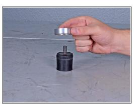
• Lift the isolator cup straight off of the isolator to remove it.
