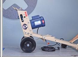
• Tilt the device back to rest on its handle.
