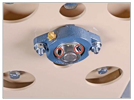
Use a 1/8 inch hex key to loosen the two set screws on the lower flange bearing.
