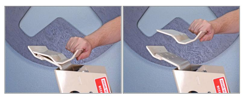
Remove the blade retainer.
