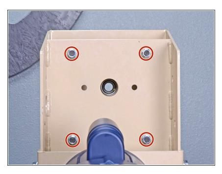
Use a 9/16 inch socket to remove the four nuts securing the isolators to the frame.
