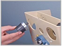
Remove the four isolators by pulling them out through the holes in the bottom of the frame."
