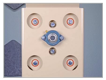
Use a 9/16 inch socket to remove the four bolts securing the striker plate to the isolators.
