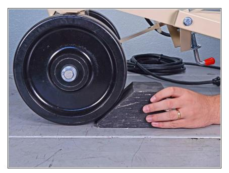
Insert wheel chocks behind the wheels to ensure the device does not move or fall during the repair."
