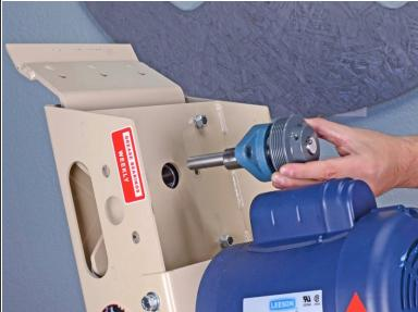
Remove the cam shaft assembly
