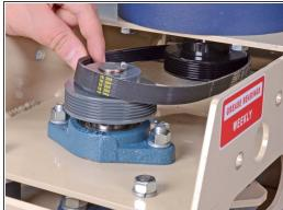
Remove the belt from the cam shaft pulley.
