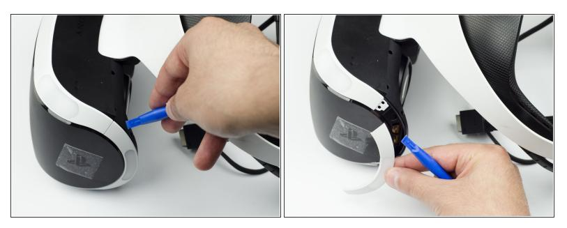
Using the plastic opening tool, carefully pry the white plastic panel free from the side of the headset. Repeat this action for the opposite side.
