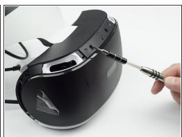
Unscrew the two 7 mm screws from the top of the headset.
