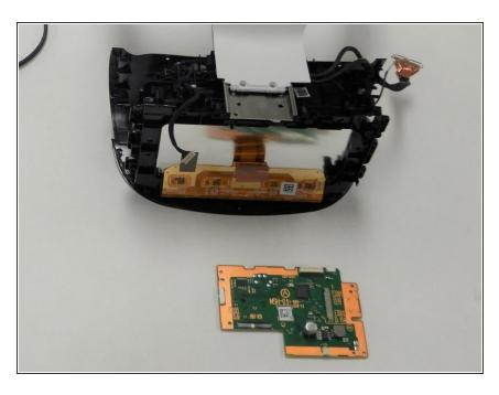
Carefully remove the motherboard and place it on a hard dry surface.
