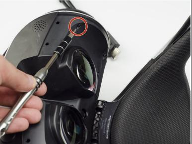
Unscrew four 13 mm screws with a PH #000 screwdriver.
