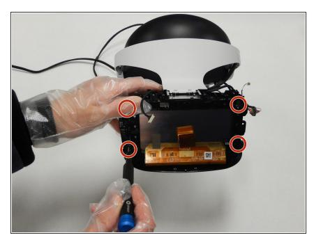
Remove the four 6mm screws holding the display in place using the Phillips #000 screwdriver.
