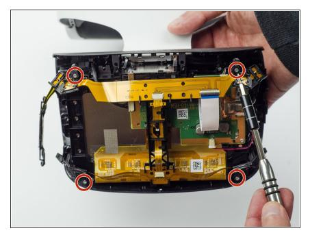
Unscrew the four silver 6 mm screws in each corner using a PH #000 screwdriver.
