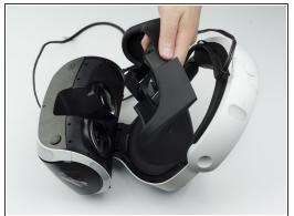
Peel back the rubber covering around the lenses to remove the surrounding plastic eyepieces.
