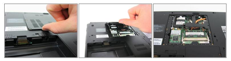
• Use a finger to remove the panel by lifting up on the provided removal tab.
