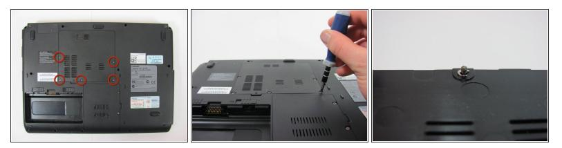
• Remove the 5 Phillips screws holding the panel in place.
