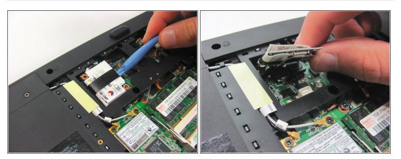
Using a plastic removal tool, dislodge the modem. This separates a small connections on the underside of the modem.
