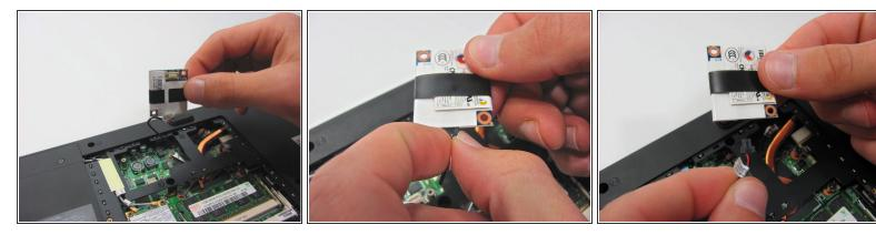
Grab the black insert connected to the modem. Gently pull the insert outwards to disconnect the cable.
