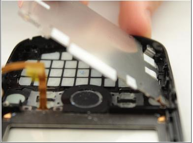
• The metal plate should now be loose enough to where one can remove the metal plate with either the plastic opening tool or with one's hands. Remove the metal plate and the keyboard beneath it can be easily removed.
