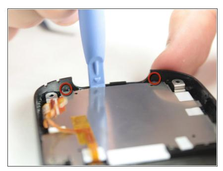
• Insert the plastic opening tool between the metal plate and the bottom of the phone as shown. Note that for this step, inserting the plastic opening tool between the two circled tabs as shown will remove the plate from both of the tabs.
