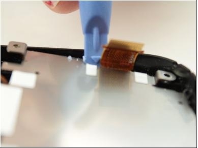
Insert plastic opening tool as shown and lift up to dislodge plate from tab.
