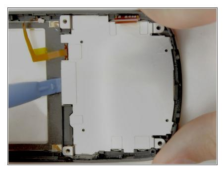
Insert plastic opening tool as shown and lift up to remove from tabs. You should hear a 'pop' and then feel the plate become loose.
