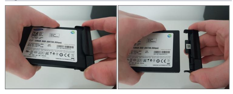
• Dislodge the caddy from the drive by lifting the caddy up and wiggling it outwards at the same time.
