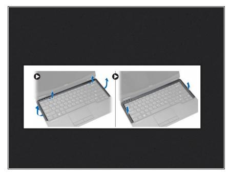
• Using a plastic scribe, pry the keyboard trim to release it from the computer. Lift up to remove the keyboard trim from the computer.
