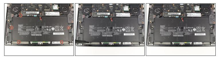
• Remove the five 3.6 mm screws from the battery with a Phillips #00 screwdriver.
