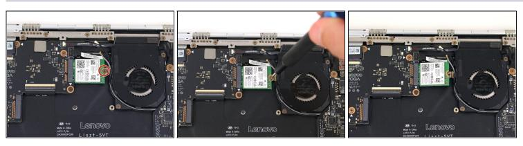
• Using a Phillips #00 screwdriver, remove the 2.2 mm screw holding down the Wi-Fi card.
