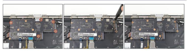
• Remove the five 3.6 mm screws from the motherboard using a Phillips #00 screwdriver.
