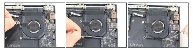
• Unwind the black and white coaxial cables from the hooks on the right fan casing.
