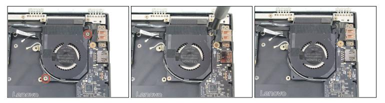
• Remove the two 3.6 mm screws from the right fan using a Phillips #00 screwdriver.
