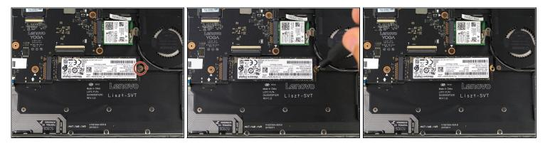
• Use a Phillips #00 screwdriver to remove the 2.7 mm screw that is holding down the SSD card.
