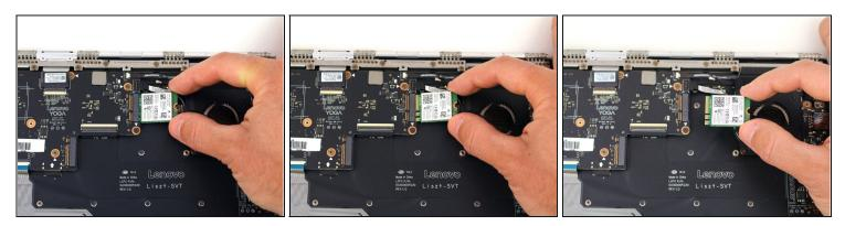
• Pull the WiFi card out from the connector on the motherboard.
