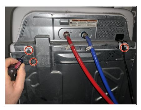
Use a 1/4-in Flathead screwdriver to remove the three 5mm screws behind the washing machine.
