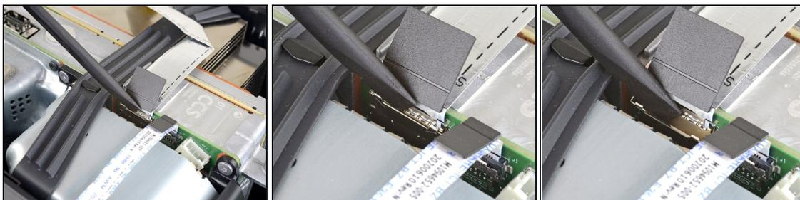
⚠ The ribbon cables and their connectors are extremely fragile, so always open locking tabs gently and pull cables slowly.
