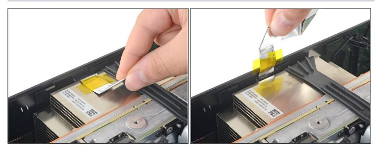
• Gently peel the taped USB port ribbon cable off of the heatsink.
