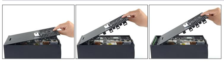
(i) The back panel slots into a gap at the top of the shell.
