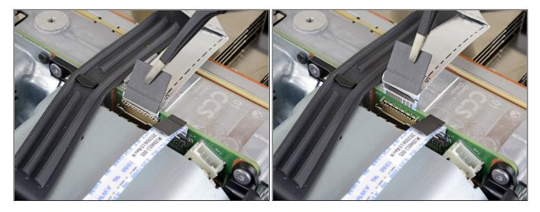
• Use a pair of tweezers to pull up on the black plastic pull tab to disconnect the USB port cable.
