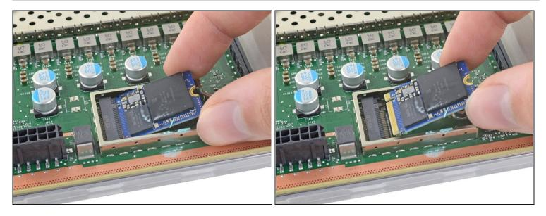
(i) With the SSD screw removed, the SSD will pop up at a shallow angle.
