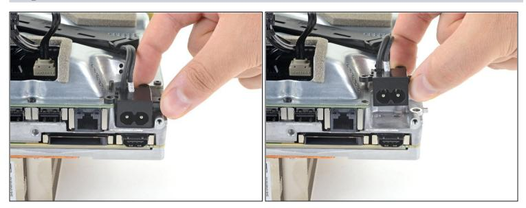
• Lift the power connector out of its recess in the chassis.
