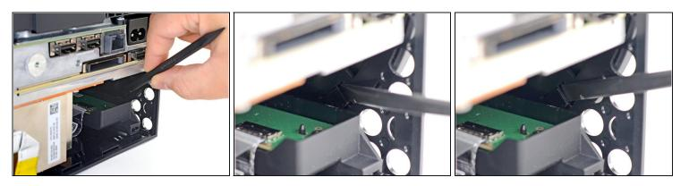
• Use the flat end of a spudger to lift up on the locking tab holding the base to the shell.
