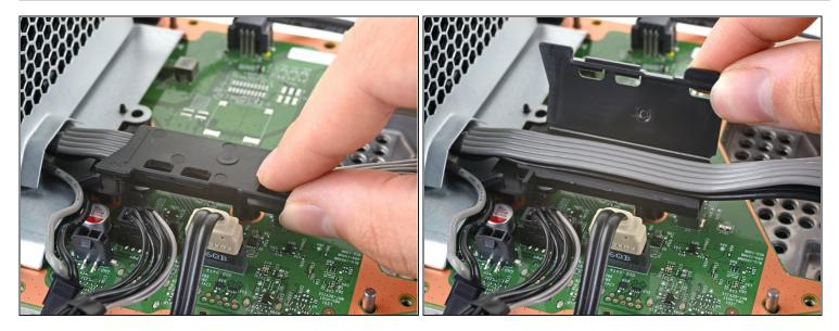
• Open the lid on the power supply's plastic cable guide.
