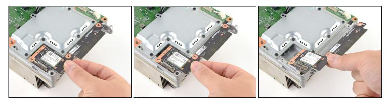
• Grip the antenna board and pull it directly away from the center chassis to disconnect it.
