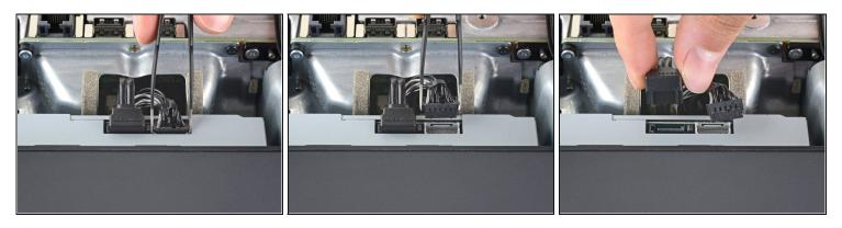
Use a pair of blunt tweezers to grip the edges of the optical drive power connector and pull up to disconnect it from the optical drive.
