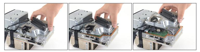
• Lift up the board shield to remove it from the center chassis.
