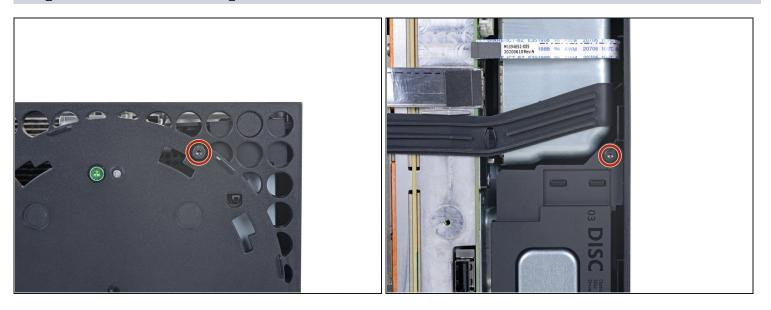
• Use a T8 Torx driver to remove the two 8.8 mm screws securing the optical drive's vibration isolator to the shell: one on the base and one on the top of the isolator.
