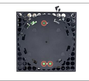
Use a T8 Torx driver to remove the three 7.4 mm screws securing the center chassis assembly to the shell.
