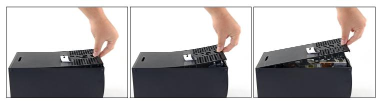
• Grip the back panel at the opening you just created and pull it up and away from the shell to unclip the long edges.
