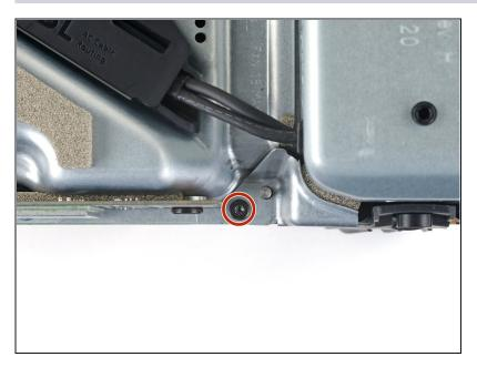
• Use a T8 Torx driver to remove the 8.8 mm screw securing the power supply corner cover.
