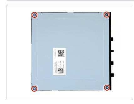
Use a Phillips screwdriver to remove the four 3.6 mm screws securing the optical drive cover.
