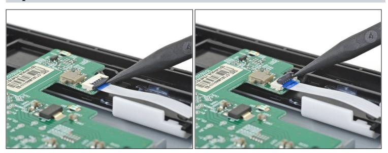
• Use the pointed end of a spudger to flip up the hinged locking tab on the small ribbon cable's ZIF connector, near the corner of the optical drive.
