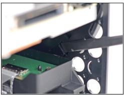
Use the flat end of a spudger to lift up on the locking tab holding the base to the shell.
