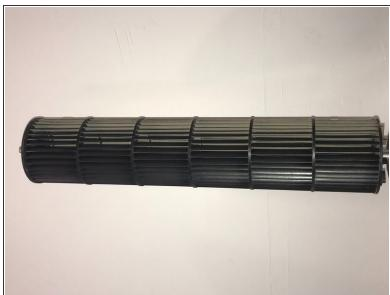
Remove the two 5 mm screws holding the fan blade in place using the Phillips #1 screwdriver.
