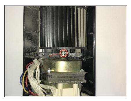
Remove the single 5 mm screw between the fan blade and the motor using the Phillips #1 screwdriver.
