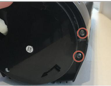
Remove four 5 mm screws from the sides of the base of the fan using the Phillips #1 screwdriver.
