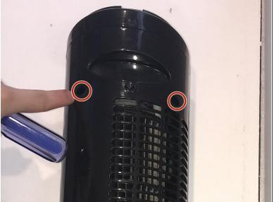
Remove the two 5 mm screws located on the outside of the case inside the holes using the Phillips #1 screwdriver.
