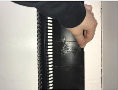
• Pinch the sides of the case to remove the case from the rest of the fan.
