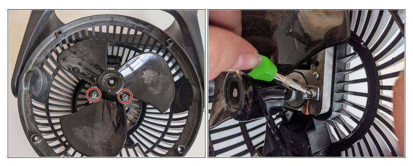
Use a Y000 tri-point screwdriver to remove the two screws from under the fan blades, turning counterclockwise.
