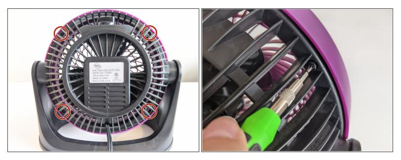
Use a Y000 tri-point screwdriver to remove four screws from the backside of your the fan, turning counterclockwise.
