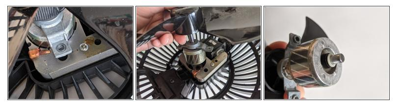
• Carefully remove the fan blades by holding the base and lifting it up out of the motor.
