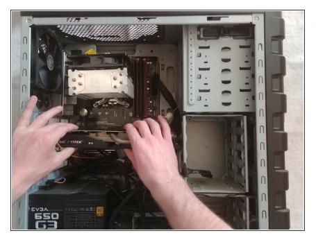
Remove the GPU from the case. If it does not move, check to make sure that steps 3-5 were properly performed.
