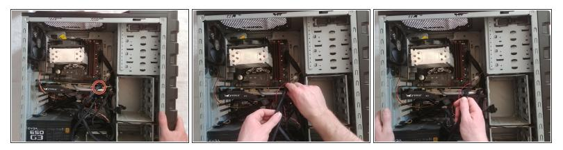
Pinch the lock at the end of the GPU power cable and carefully disconnect it.
