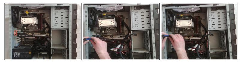
• Remove the two Philips #1 mounting screws that attach the GPU to the inside of the case.
