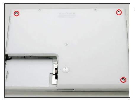
Remove the three newly-revealed Phillips screws.
