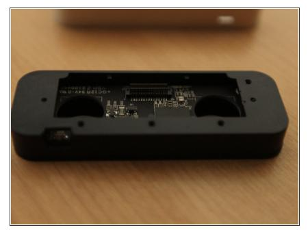
• Peel back the tape on the internal components and lift the lenses out.
