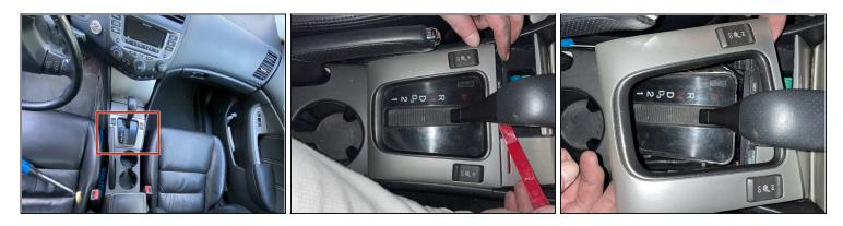
• Remove the shifter frame panel with the same opening tools.
