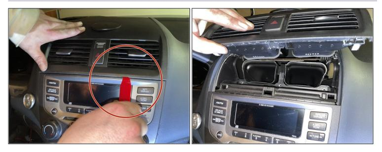
• Remove the center climate vents with the opening tools.
