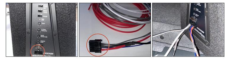
Attach the wiring harness into the amp by clipping it in.
