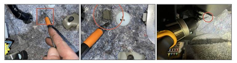
• Drill a hole through the firewall located on the foot well of the driver's side under the steering wheel.
