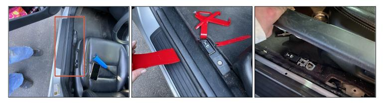
Use the plastic opening tools to remove the floor trim panel on the driver's side door.
