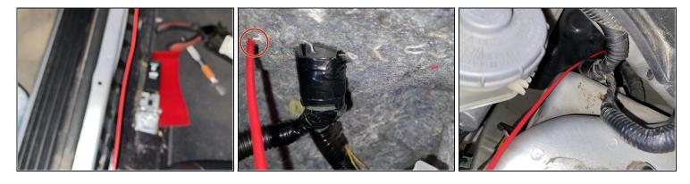
• Run the power and ground wires from the trunk through the door sill and through the firewall to the engine bay.
