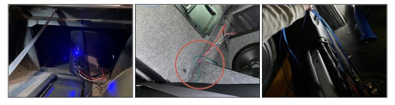
• Run the wires under the back seat and along the driver's side door sill (removed in step 1) to under the steering wheel.
