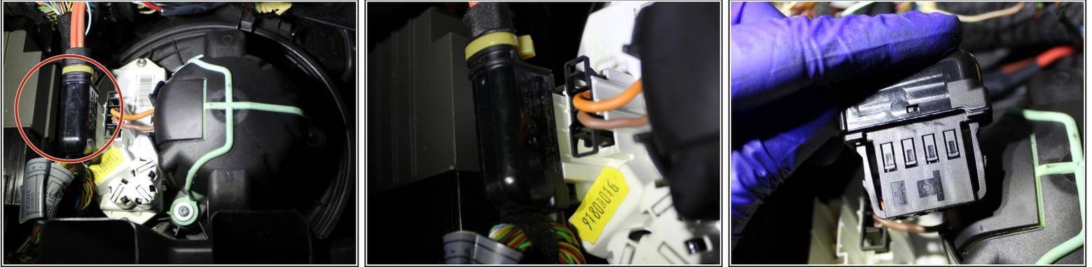
**i** There is only one connector that needs to be disconnected to remove the blower motor. This connector is black with two red/orange wires going into it.
