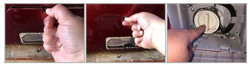
• Jiggle the water filter compartment while pulling it towards yourself to remove the compartment.
