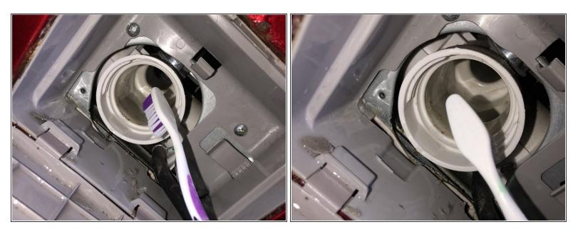
• Use the toothbrush to clean the slot in the washing machine where the water filter is inserted.
