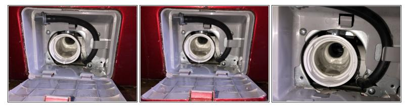
Inspect the inside to make sure there is no leftover lint or unnecessary objects that can clog the water filter.
