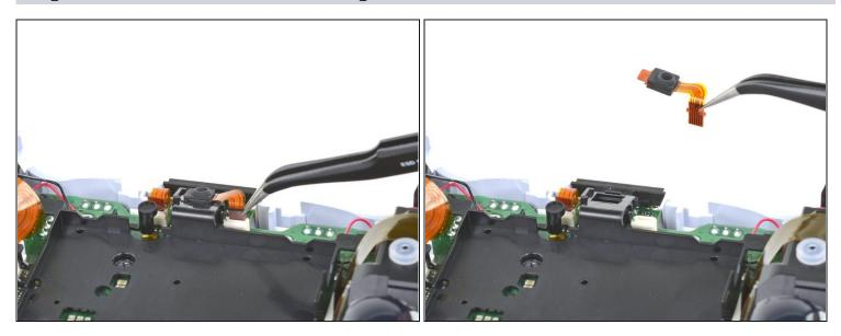
• Grab the lower microphone ribbon cable pull tab with your fingers or a pair of tweezers and disconnect it from the motherboard.
