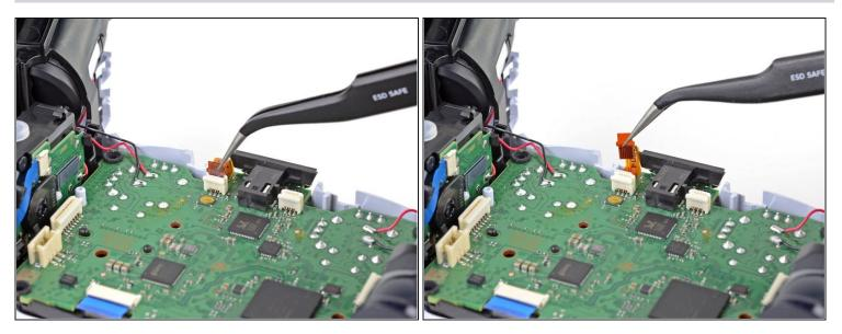
• Use a pair of tweezers or your fingers to grip the upper microphone ribbon cable pull tab, and pull up to disconnect it from the motherboard.
