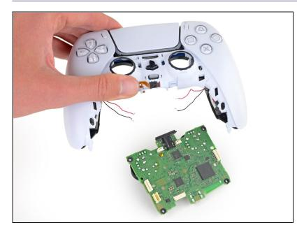
• Separate the controller from the motherboard.
