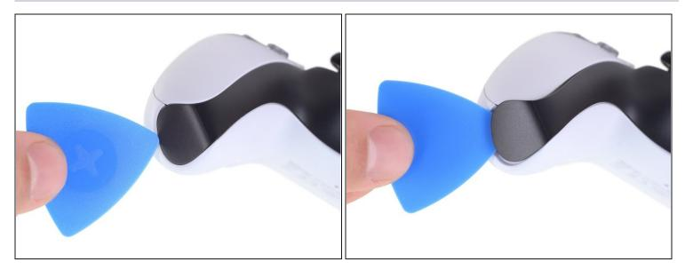
• Insert an opening pick underneath the middle trim at the bottom-left corner of the controller to release the clips securing it to the case.
