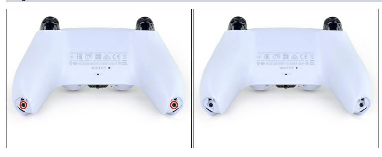
• Use a Phillips screwdriver to remove the two 6.4 mm screws securing the bottom corners of the lower case.
