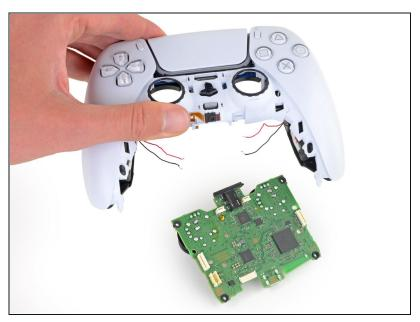
• Separate the controller from the motherboard.
