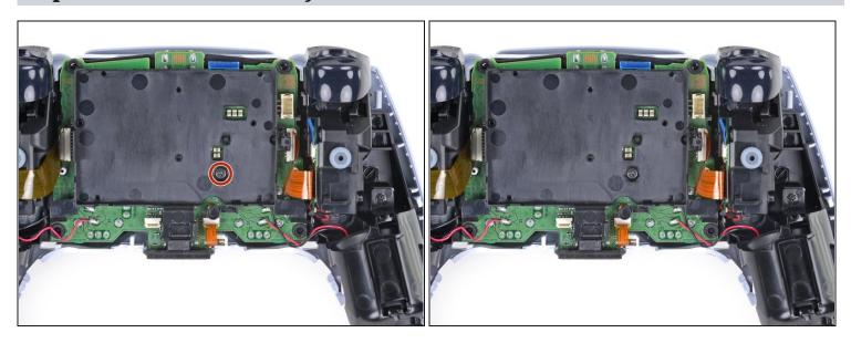
• Use a Phillips screwdriver to remove the 6.4 mm screw securing the battery bracket.
