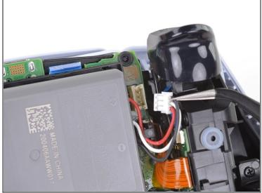
Use a pair of tweezers or your fingers to disconnect the battery from the motherboard.
