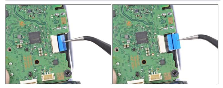
• Use a pair of tweezers or your fingers to grip the touchpad ribbon cable pull tab, and pull it straight out of the motherboard connector.
