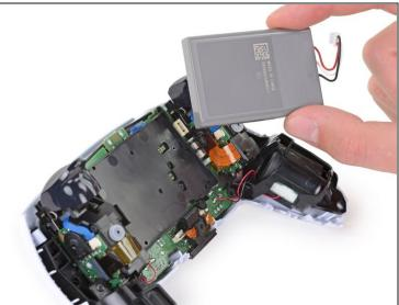
Lift the battery straight out of the battery bracket.
