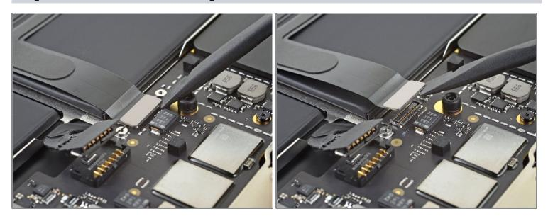
• Use the flat end of a spudger to pry the trackpad cable connector up and out of its socket.
