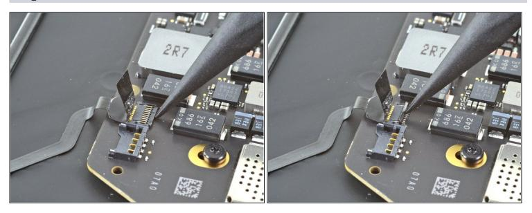
• Use the pointed end of a spudger to lift up the small locking flap on the microphone cable's <u>ZIF connector</u>.
