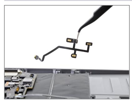
• Remove the microphone array.
