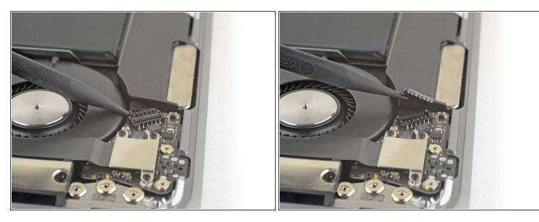
Slide the pointed end of a spudger underneath the speaker cable and pry straight up to disconnect it.
