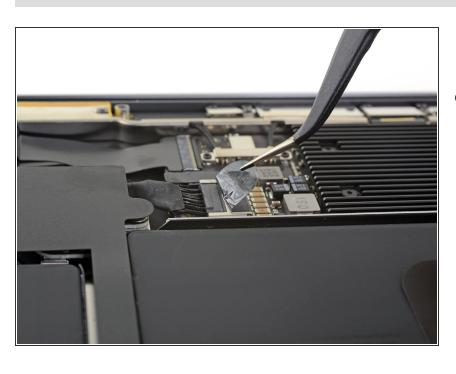
Peel back the tape covering the battery connector enough to reveal the connector underneath.
