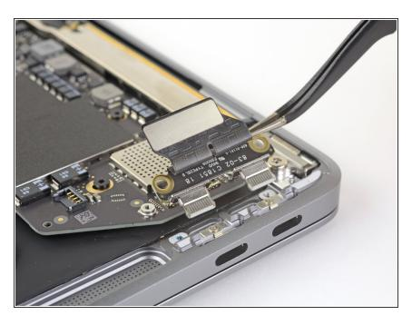
Use a pair of tweezers to remove the USB-C board. Compare your new replacement part to the original part—you may need to transfer remaining components or remove adhesive backings from the new part before installing.
