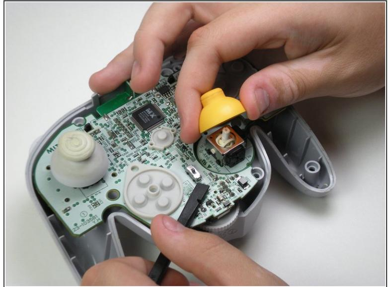
**⚠ Potential for device damage: Rough handling of the C-stick could cause the daughterboard to break off of the motherboard.**
