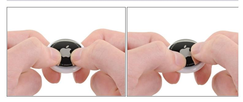
• Rotate the battery compartment door counter-clockwise to unlatch it from the frame.
