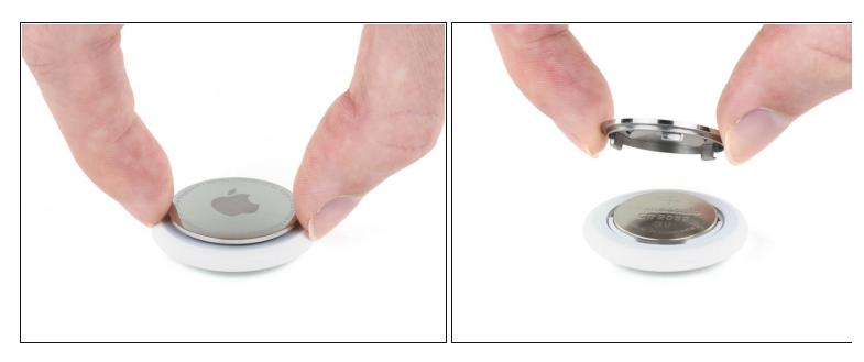
• Lift up the battery compartment door to remove it.
