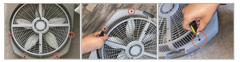
Use the Phillips #0 screwdriver to remove four 8.8 mm screws that are marked on the back of the grill.
