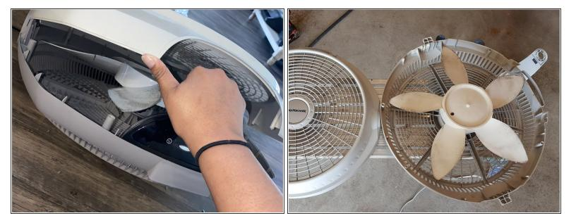
• Unlatch the top of the fan to separate the grill and reveal the blade.
