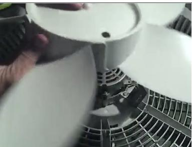
Grab both sides of the blade and twist counter clockwise to remove it from the base axel attached to the back grill.
