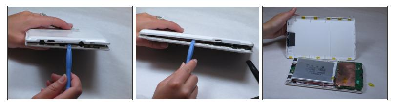
Remove the back panel by using the plastic opening tool to carefully pry around the panel's edges.
