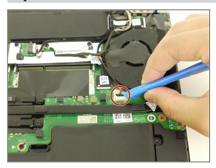
Disconnect the fan and heatsink assembly from the motherboard using the plastic opening tool.
