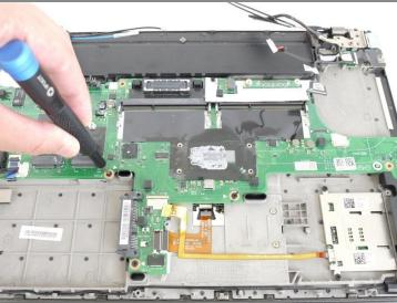
Using the JIS #00 screwdriver, remove six 2.8 mm screws securing the motherboard to the device.
