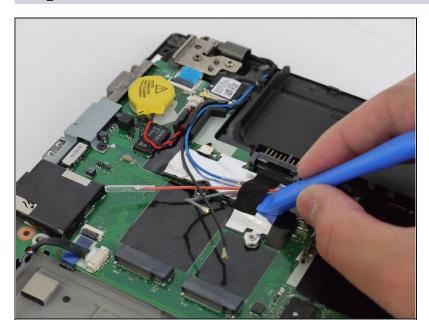
Use the plastic opening tool to remove the black piece of tape holding the cables together.
