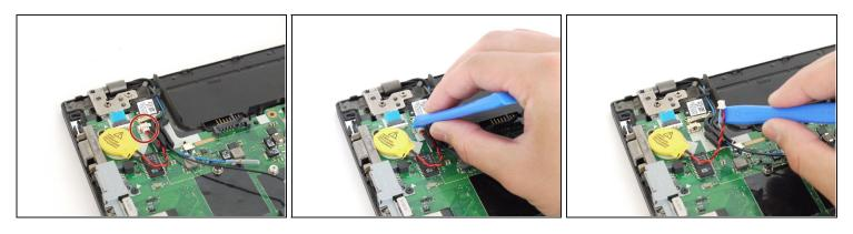
• Using the plastic opening tool, disconnect the CMOS battery from the motherboard.
