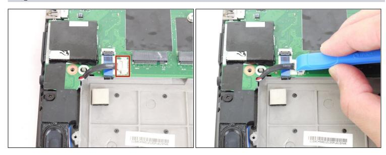
• Disconnect the speaker cable from the motherboard using the plastic opening tool.
