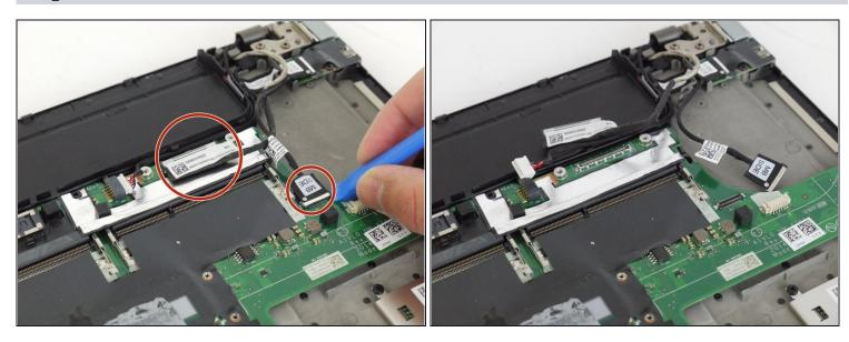
Disconnect the daughterboard cable and the display cable using the plastic opening tool.
