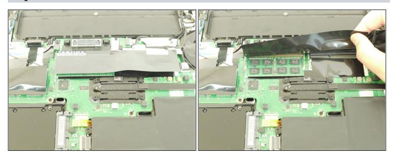
• Lift up the black piece of tape and remove it to uncover the RAM sticks underneath.
