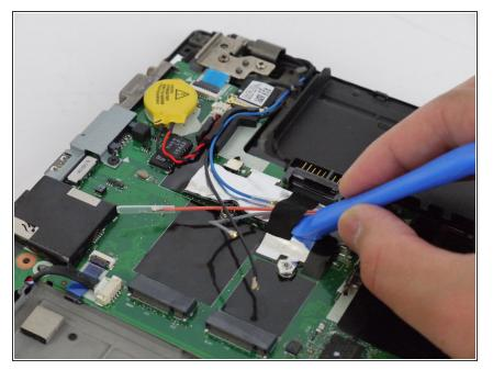
• Use the plastic opening tool to remove the black piece of tape holding the cables together.
