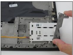
• Remove the smartcard reader bracket from the device.
