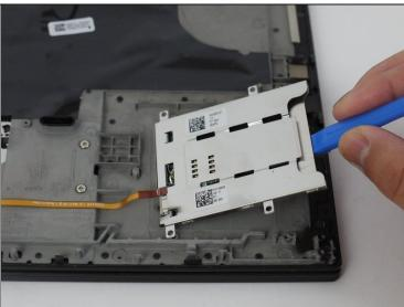
• Lift up the smartcard reader and remove it from the device.
