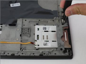
• Using the JIS #00 screwdriver, remove the four 2.8 mm screws securing the smartcard reader and bracket to the device.
