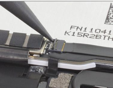
Use the pointed end of a spudger, an opening tool, or your fingernail to flip up the small, hinged locking flap on the home button assembly <u>ZIF connector</u>.
