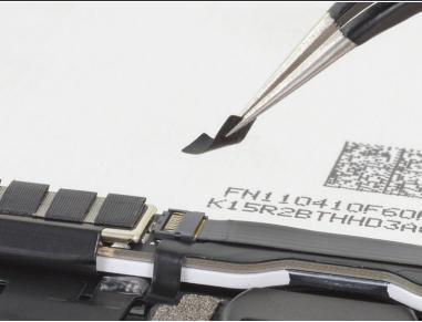
• Use a pair of tweezers to remove the sticker covering the home button assembly ZIF connector.
