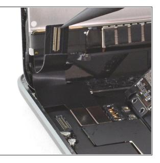
Use the pointed end of a spudger to disconnect the digitizer press connector from the logic board.
