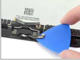
Use an opening pick to continue separating the home button assembly cable from the screen.
