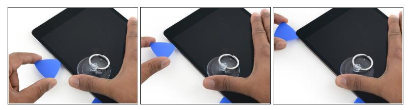
Slide the opening pick around the top left corner of the iPad to separate the adhesive.
