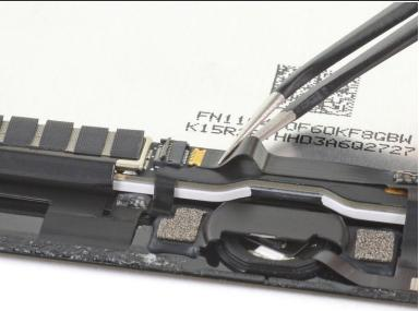
Use a pair of tweezers to pull the home button assembly cable out of the ZIF connector.
