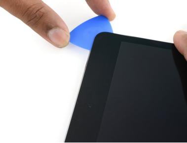
• Insert the previous pick deeper into the iPad and slide it away from the camera toward the corner.
