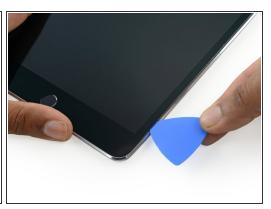
Continue sliding the opening pick down the right edge of the iPad, reheating the edge using an iOpener if necessary.
