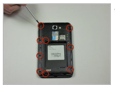
Remove the nine 3mm screws on the perimeter of the phone with a Phillips #00 screwdriver.
