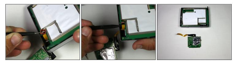
• Use the tweezers or the spudger to lift the tan latch off the ribbon cable (ZIF connector) and gently pull out the ZIF connector and cable from underneath the opened latch.
